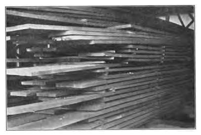
Fig. 67.—Badly warped boards. The trouble here is due to a poor arrangement of stickers and to the piling together of boards of unequal length.
